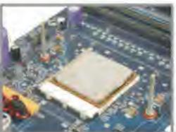
Apply a thin layer of included thermal compound onto the processor.
